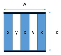
Figure 1 – Capacitor cross-section with specifications of w=1 mm, X section: er=4, width = 20% of w; Y section: er=1 and width= 20% of w, Assume length: L=1mm
